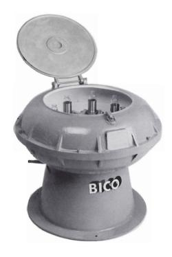
The **BICO OIL CENTRIFUGE** is designed for maximum safety, from the explosion proof motor to the optional explosion proof starting switch. The cast aluminum door atop the high tensile cast iron housing forms an almost completely airtight chamber.
